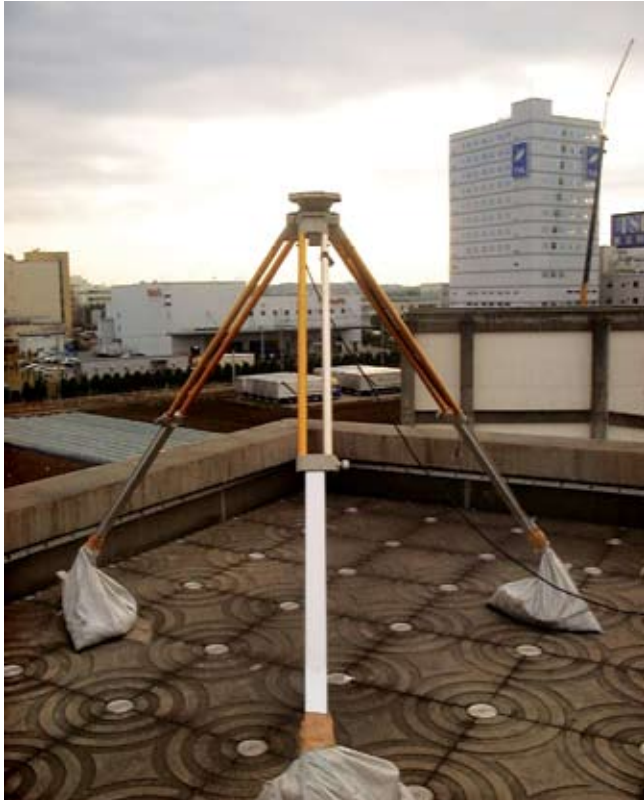
The antenna for the GPS reference receiver (upper left photo), the tower site of the GPS rover receiver (upper right), and a schematic diagram of the overall installation.
